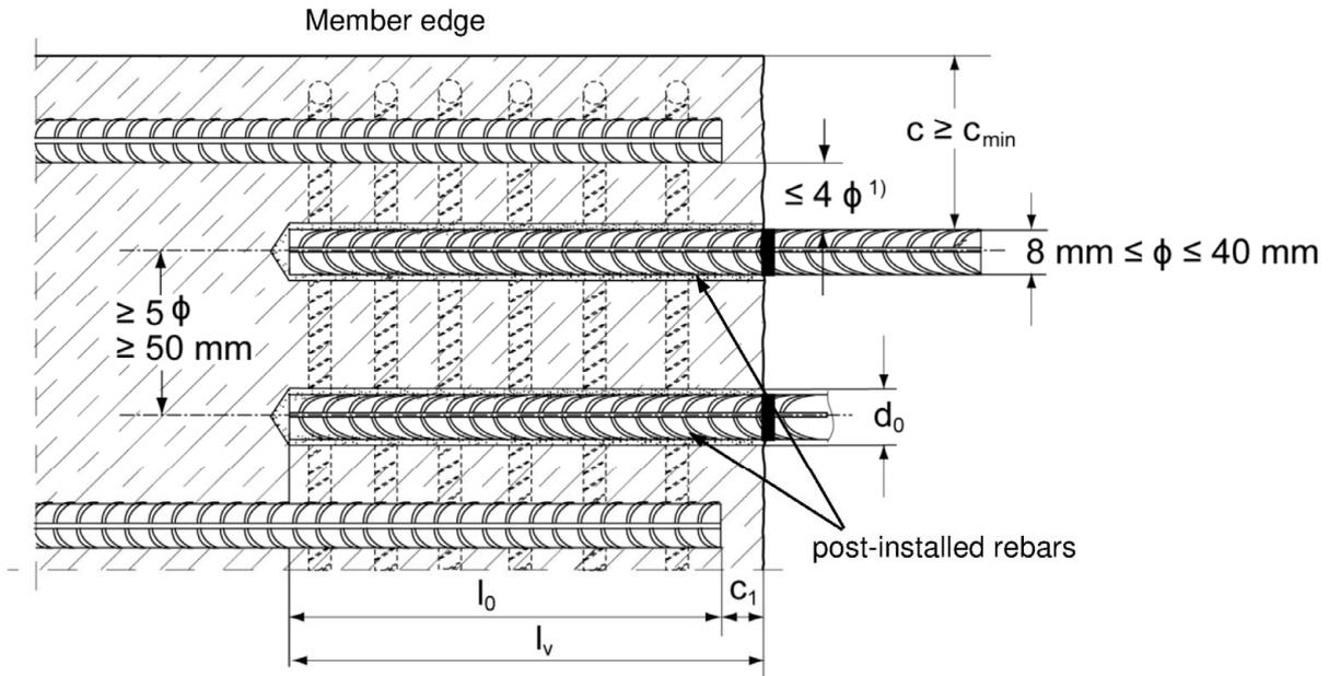
1) If the clear distance between lapped bars exceeds  $4\phi$  then the lap length shall be increased by the difference between the clear bar distance and  $4\phi$
