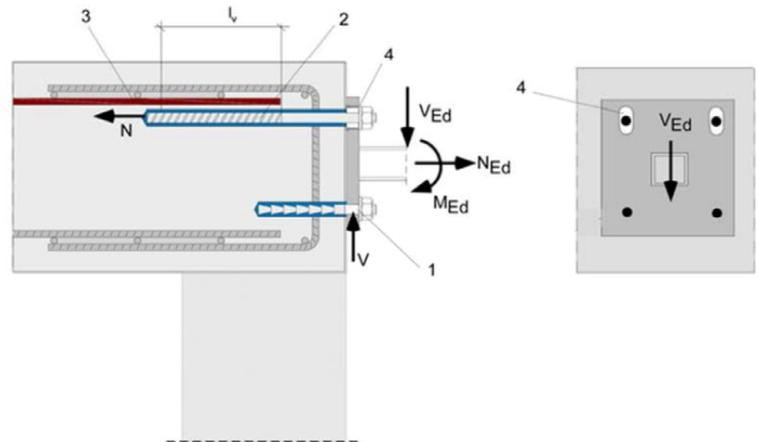
The required transverse reinforcement acc. to EN 1992-1-1:2004+AC:2010 is not shown in the figures. **The fischer rebar anchor may be only used for axial tensile force.** The tensile force must be transferred by lap to the existing reinforcement of the building. The transfer of the shear force has to be ensured by suitable measure, e.g. by means of shear force or anchors with European Technical Assessment (ETA).
