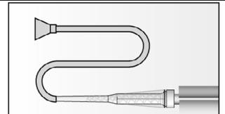
Assemble mixing nozzle FIS MR Plus or FIS UMR, extension tube and appropriate injection adapter (see **table B4.3**)
