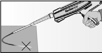
Press out approximately 10 cm of mortar until the resin is permanently grey in colour. Mortar which is not grey in colour will not cure and must be disposed.
