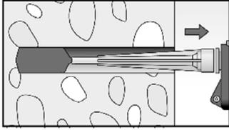
Inject the mortar from the back of the hole towards the front and slowly withdraw the static mixer step by step with each trigger pull. Avoid bubbles.
