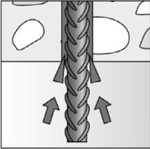
For overhead installation, support the rebar and secure it from falling till mortar started to harden, e.g. using wedges.
