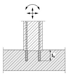
Figure A1.2: Slab / beam to wall or beam to column
